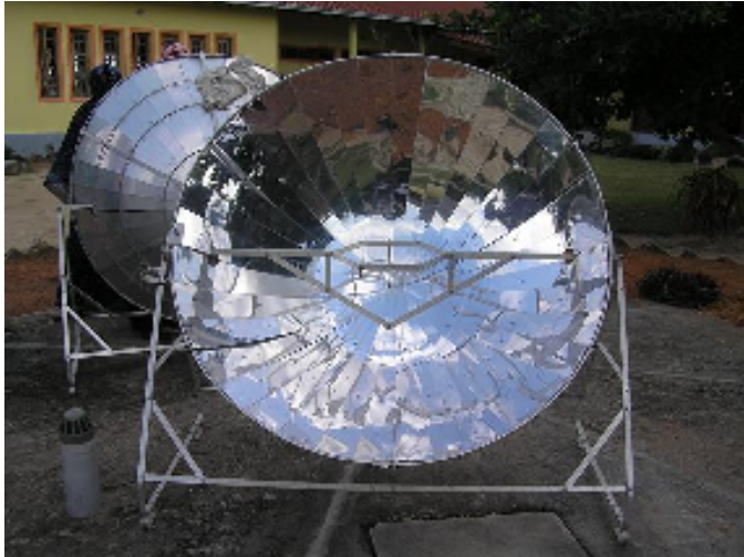
Figure 10 Solar parabolic concentrating cooker SK 14
